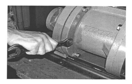
C. Remove the casing bolts (104-3); leave the two (2) disassembly/assembly bolts (104-58) in the tapped holes on either side of the bracket (028). Use these bolts to separate the bracket (028) from the casing (001) (photo 3).
