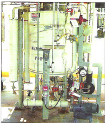
The Magnatex® pump operates without cavitation, despite only 2 ft of NPSH.
