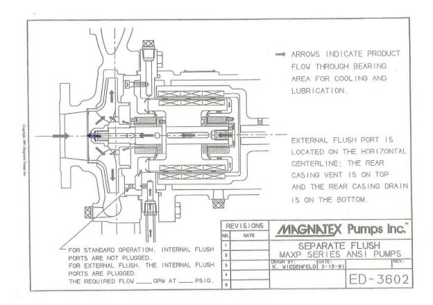
Connect the separate flush piping to the  $\frac{1}{2}$ " NPT flush connection located 90° to the right on the rear casing flange, as viewed from the pump suction end.
