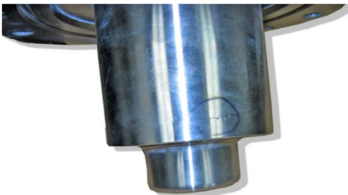
Rear casing breach caused by solids-laden vortices
