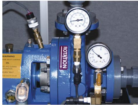
*Process pumps need gauges installed, otherwise the operator has no reference point to determine the system's health.*
